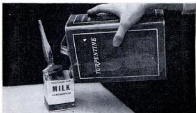
"Mopping up" after cleaning paintbrushes is simple if a disposable milk carton is used to hold the turpentine or thinner
